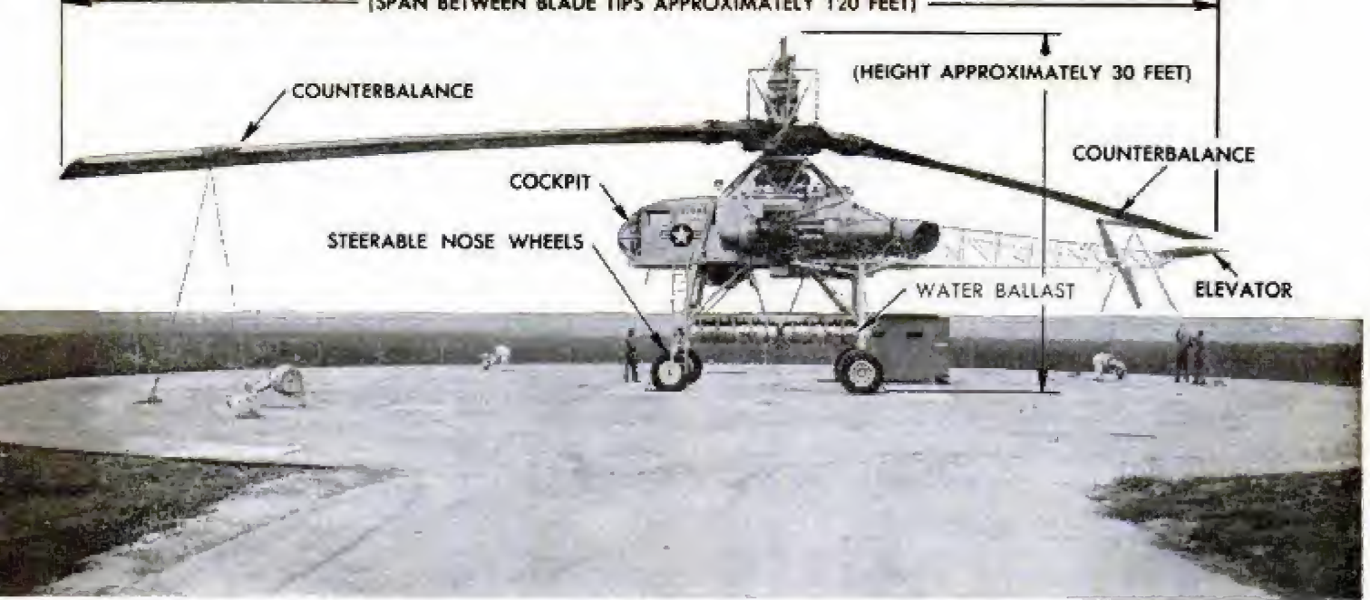
Tied down during ground tests, the huge XH-17 dwarfs near-by workers. During earlier experiments it broke loose from its moorings and was slightly damaged
